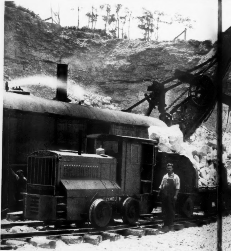
Plymouth 8-ton Locomotive at Gibsonburg (O.) Quarry of The William L. Wood Lumber Co.
